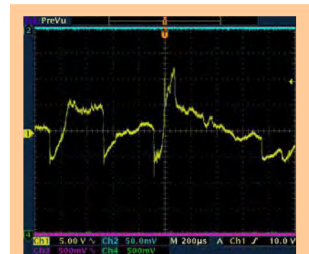
Standard Arc Power Supply Fluctuation ( \pm 10 V)
